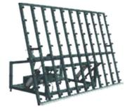
Designed to pneumatically tilt to a vertical position, facilitating the transfer of large single sheets in the fabrication of insulating units or the transfer of completed IG Units to carts or racks.
